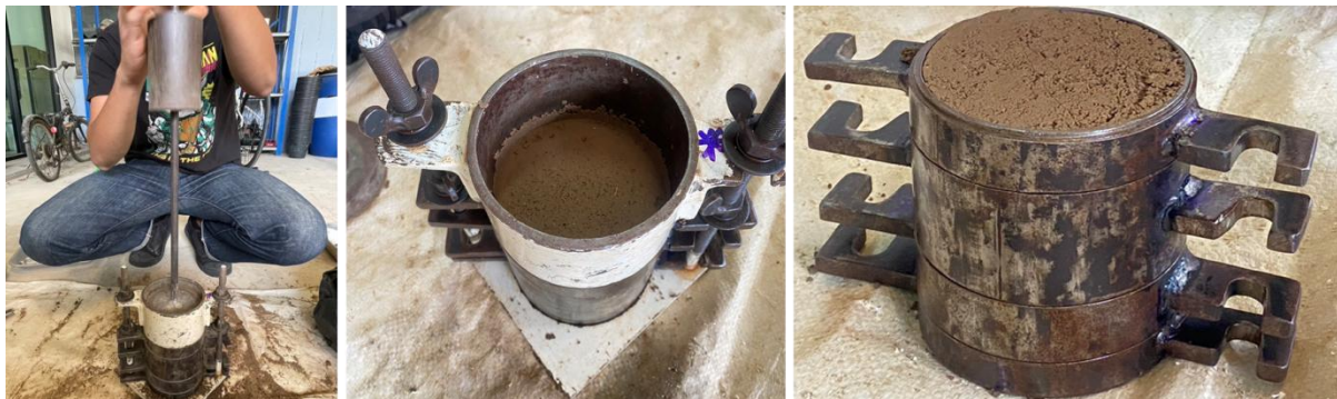
Figure 2. The compaction test conducted at energy levels of 2475, 7425, 12375, and 56000 ft–lb/ft 3
