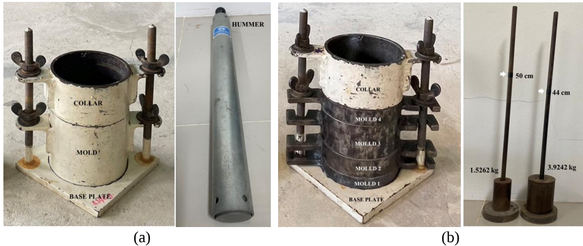
Figure 1. (a) The mold, base plate, collar, and hammer used in the Modified Proctor Test, and (b) the modified mold consisting of four sections: 2 cm, 2.50 cm, 5 cm, and 2.15 cm, along with two sets of hammers.
